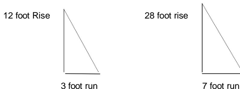
NOTE: The rise is determined by measuring the distance from the base of the structure to the point where the ladder is resting. The run is determined by measuring from the base of the structure, horizontally to the base of the ladder.
